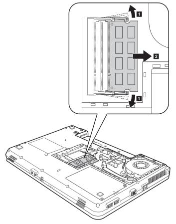
Insert the notched end of the DIMM into the socket.Press the DIMM firmly, and pivot it until it snaps into the place. Make sure that it is firmly fixed in the slot and does not move easily.
